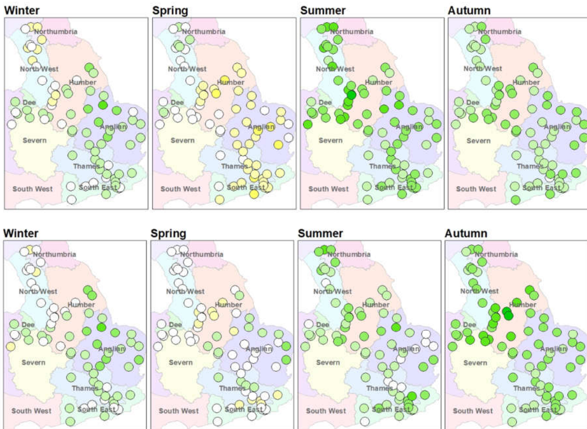
Figure 5-10 – AMO smoothed (top) unsmoothed (bottom) vs precipitation correlations across the UK. Darker shades indicating stronger positive correlations.
