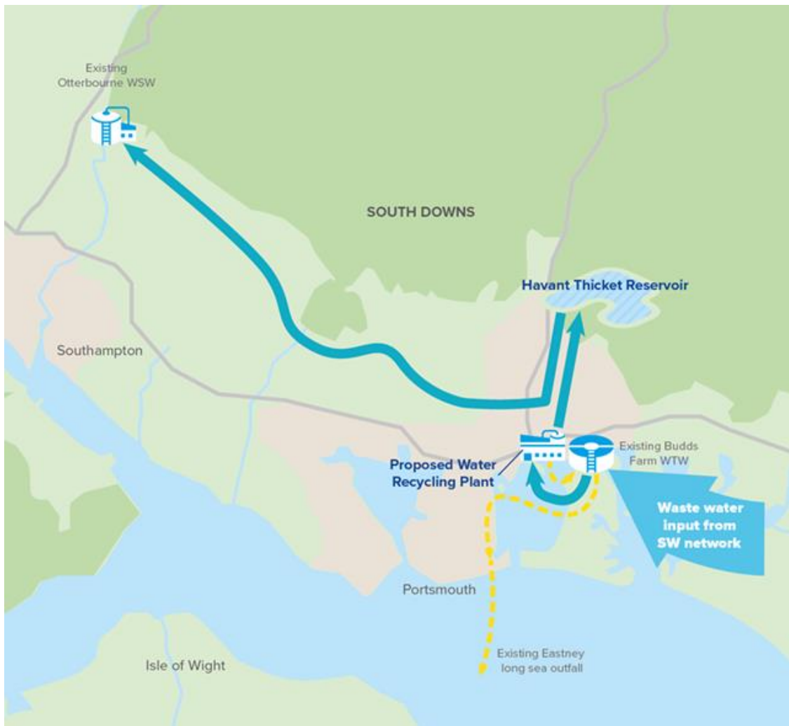
Figure 2: A schematic showing the main components of the proposed HWTWRP.
