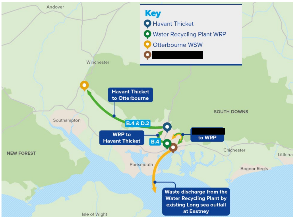
Figure 2 - Schematic of Option D.2 & B.4
