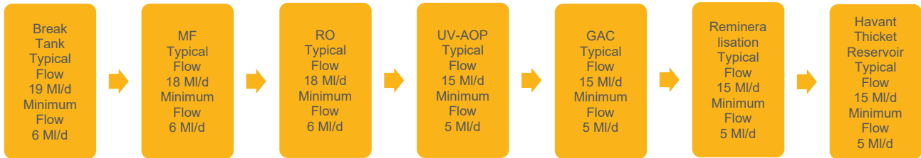
Figure 5 - Diagram showing flow leaving each process area in the WRP
